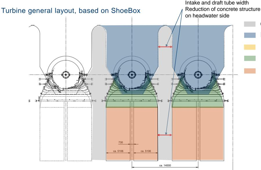
rete structure Concrete structure Intake steel liner Turbine main components Draft tube elbow steel liner
